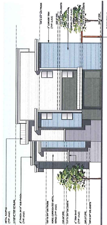
UNIT 1 UNIT 2 UNIT 3 NORTH ELEVATION SCALE: 1/8" = 1'-0"
